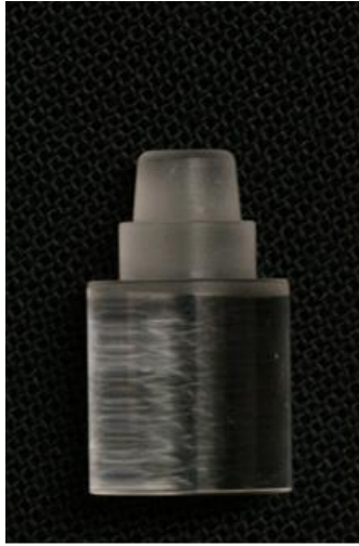
Figure 1 A standardized acrylic die with a 5-degree convergence angle and 1-mm shoulder
